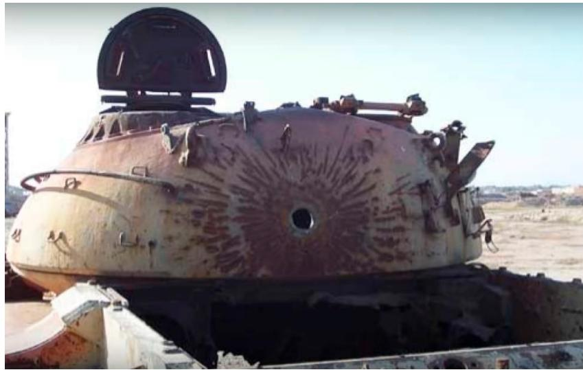
Figure 4. DU projectile penetration of tank turret. An explosive tip identifies for the gunners the point of impact.
