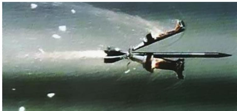
Figure 8. The sabot detaching from a depleted uranium projectile.
